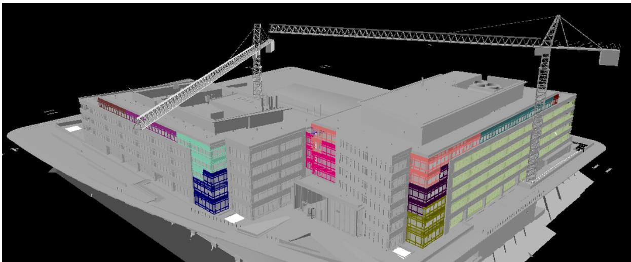
Figure 38 – Location of Prefab Glazing Panels per Delivery opposite Side
