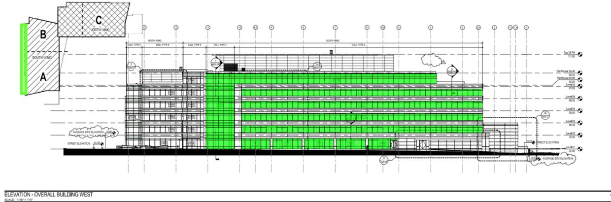
Figure 36 – Area Where Photovoltaic Glass Will be Hung for Optimum Efficiency (Drawing Courtesy of Gensler)
